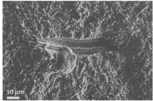
Fig. 10. The fracture-initiating flaw in a KN1 specimen, tested at 1200°C; \sigma_f = 419 MPa. The shape of the defect indicates that a textile fibre or a hair has been lying here.
